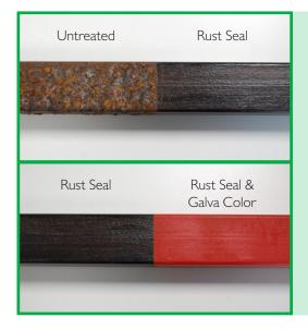
**TEST:** A rusted beam is being treated with CRC Rust Seal. On half of the treated area, CRC Galva Color is applied as a topcoat. The plate is being put in a highly corrosive salt spray cabinet for 500 hours.
